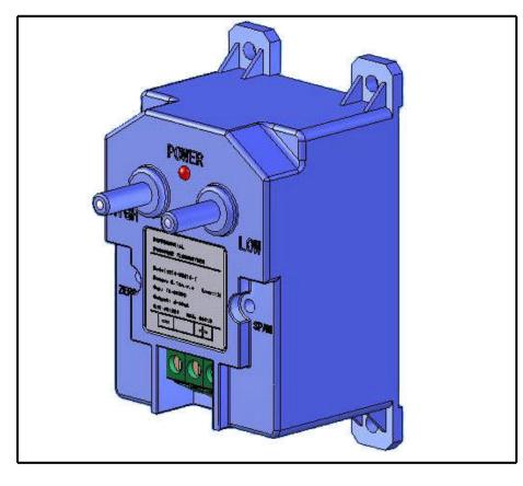
The Series 211 Differential Pressure Transmitter can accurately measure positive, negative, or differential pressure and send the corresponding 4-20 mA output signal. The Series 211 is not position sensitive and can be mounted in any orientation without compromising accuracy. It also features a power LED, so you always know when the transmitter is operating. The compact, lightweight design makes installation simple and easy.
