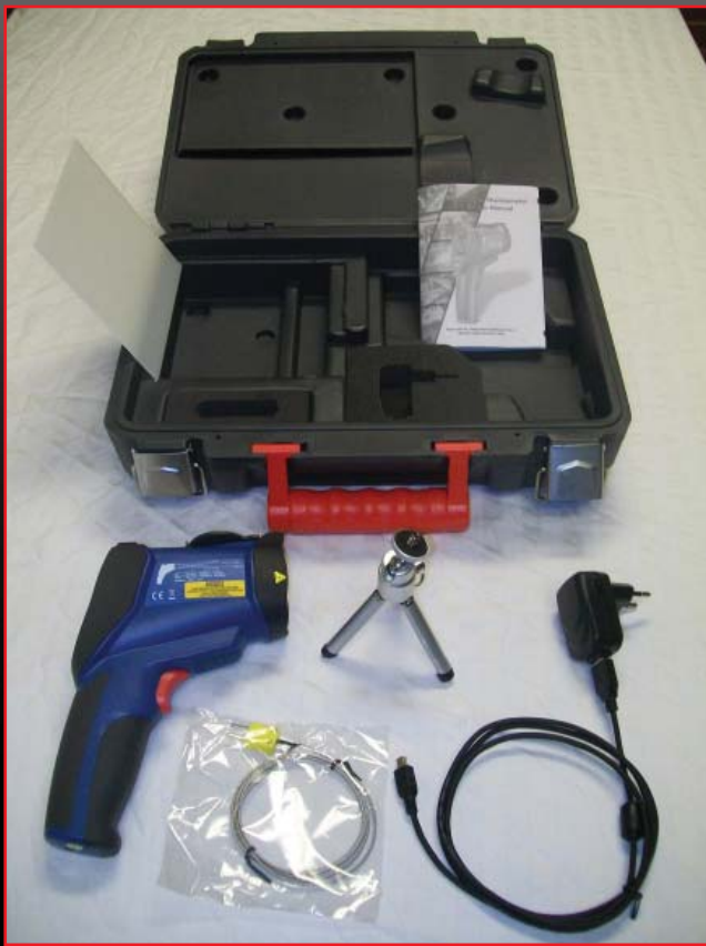
Standard Accessories: 3.7 Volt Battery, Type K Thermocouple, USB Cable, Micro SD Memory Card, Operator's Manual and Tripod, Carrying Case
