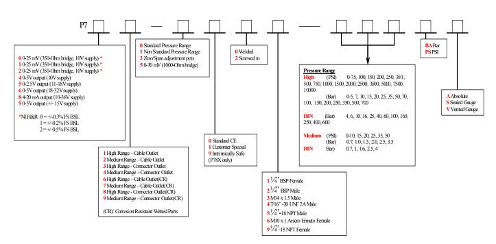
Examples: P722-0005-10PSV = 0 to 25mV output, 0.5% NLH&R, cable outlet, welded 1/4" NPT port, 10 psi vented gauge P786-0901-700BAA = 4 to 20mA output, cable outlet (corrosion resistant build), Intrinsically Safe, welded 1/4" BSP port, 700 bar absolute
