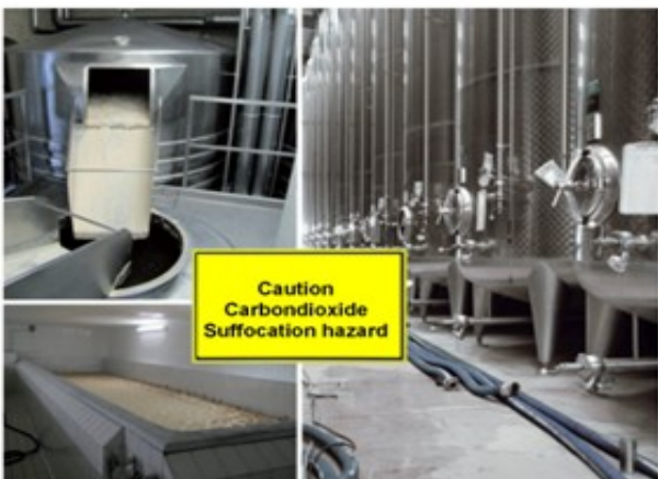
In wine cellars, breweries and the beverage industry CO 2 measurement is prescribed by law.
