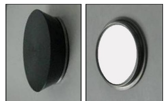
Mounted HC2-IT25 probe Left : with protection cap
